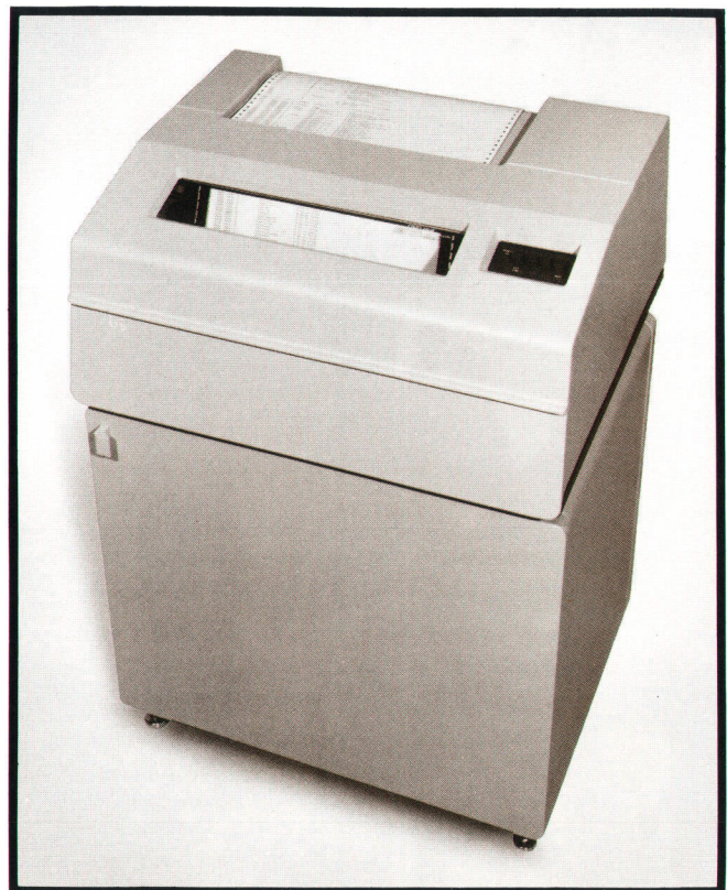
Fig. 1. Model 2608A prints 132 columns of characters on standard 14-inch wide computer paper at speeds up to 400 lines/minute when printing upper case only with a 5 × 7 dot matrix, or to 320 lpm when printing upper and lower case with a 5 × 9 dot matrix. As many as 16 different character sets can reside within the printer, any two of which may be used within any line, and the normal dot matrix can be expanded for special print characteristics. Forms with as many as six parts can be printed.
