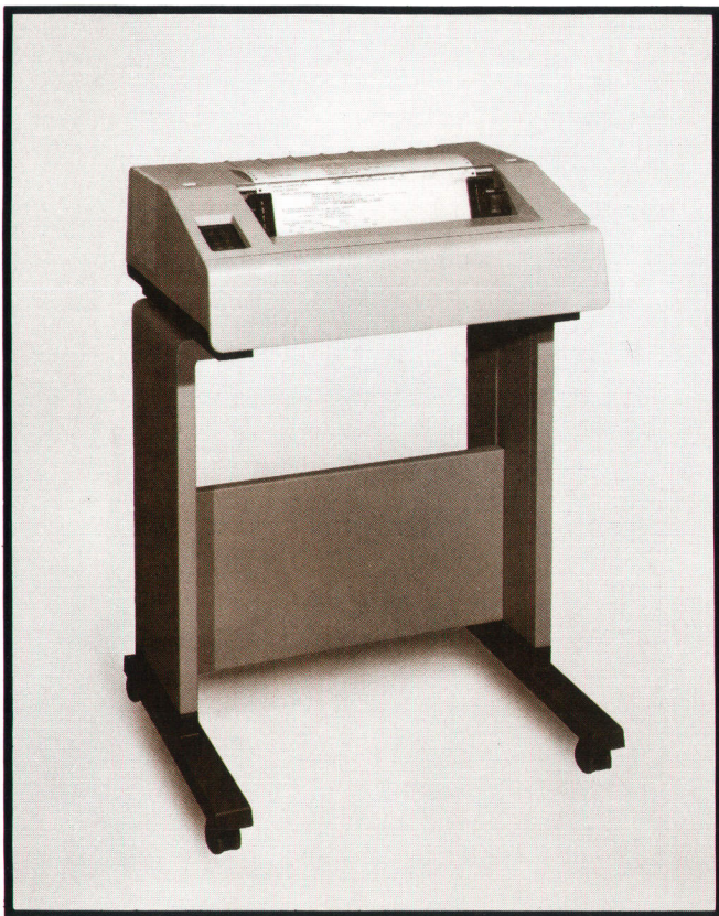
Fig. 1. Model 2631A Printer is designed for either table-top or pedestal mounting. Microprocessor control of the dot-matrix printing operation contributes to the printer's versatility while simplifying the printing mechanism. A high throughput rate is obtained with a print speed of 180 characters per second plus the ability to print in either direction and to slew past strings of blank spaces. Model 2631G, which can also print raster-style graphics, is identical in appearance.
